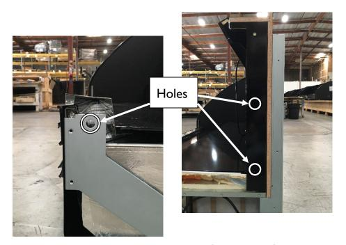
b. Install the joining bolts through the left and right frames along with washers, lock-washers, and lock nuts. The proper order for the washers as shown in the picture below is bolt, flat washer, frame, frame, flat washer, lock-nut. It does not matter which side of the center seam the nut is on.
