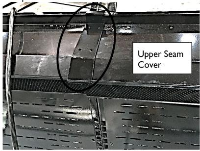
b. On the lower front of the case, the lower seam cover will be slotting behind any price tag molding (PTM) and bumper channel. The bumper channel should have the first one or two screws removed; the PTM uses double stick tape and can just be peeled back.
