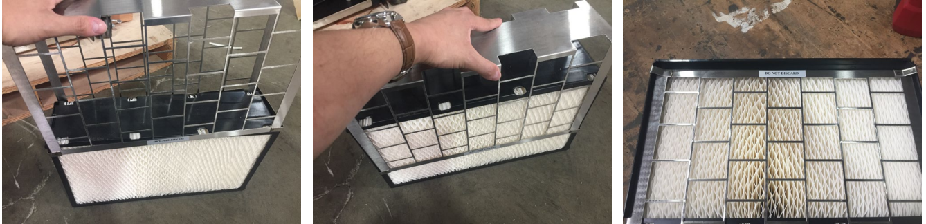
Figure 5 – Seating the new wick into the cage.
