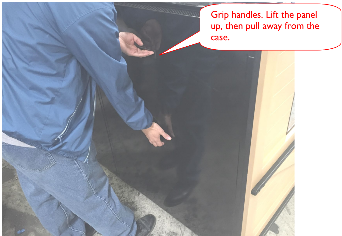
Figure 1 – Removing chimney back panel.
